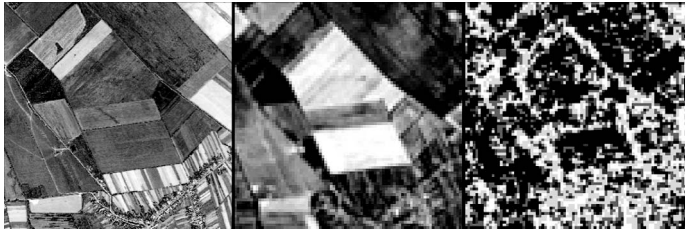
Figure 2. Example of an area characterized by heterogeneous land use pattern in high-resolution Quickbird data (left), June 2000 Landsat ETM+ data (first principal component, middle), and image texture derived from the Landsat image (first-order entropy of band 7 calculated at a window size of 3 pixels, right). The subset is centred on the village of Bezovce in Slovakia (21.15E, 48.63N).
