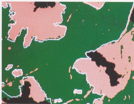
Figure 4. Classified radar image overlaped by the border of the forest land out of a forest map. Forest = green; agricultural land = sand; housing areas = black (Koch et al., page 94).
